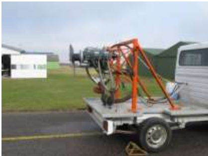
Step I: Engine placed in the test stand, and final check performed before the testrun. During test run, all necessary run-in data is captured and listed.
