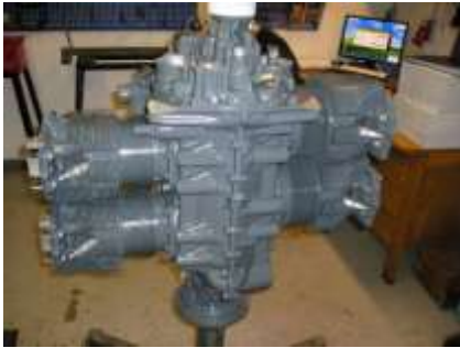
Step G: Engine ready for final assembly, after completion of painting.
