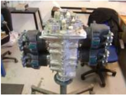
Step F: Engine being re-assembled with new factory-parts, and then primed before final painting.
